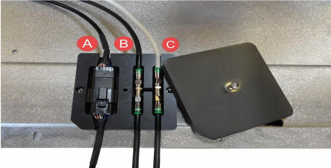
Figure 11 - Antenna Junction Box
