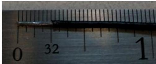
Figure 9 - Control Cable Stripped length
