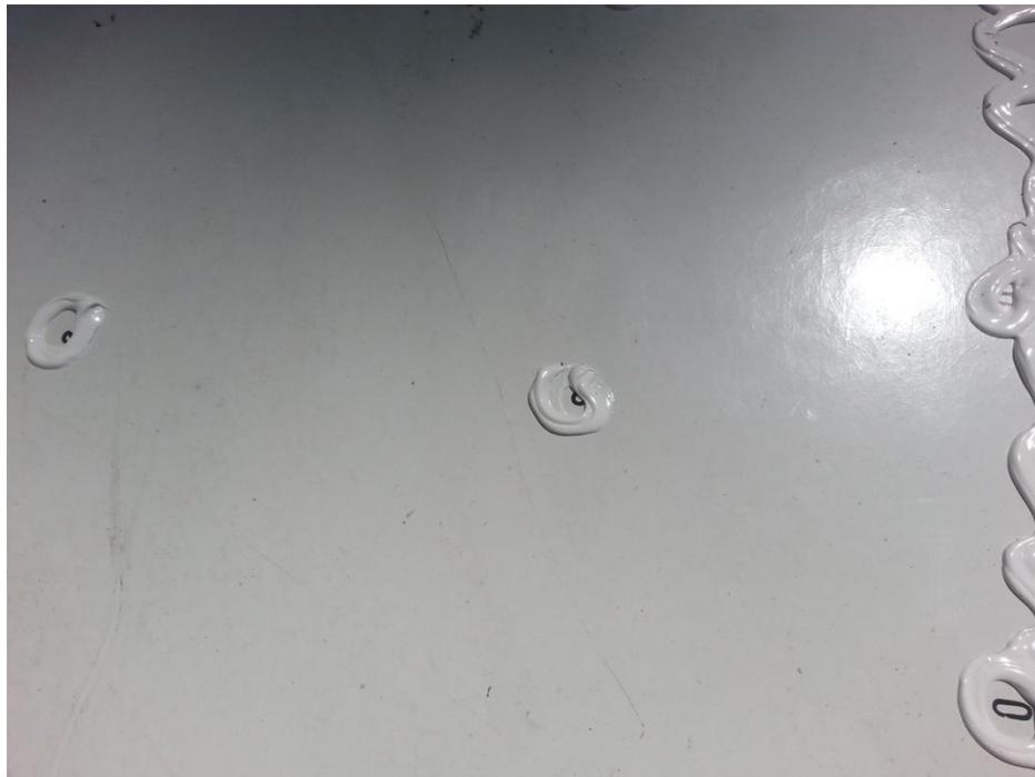
Figure 6 - Under Antenna Sealer
