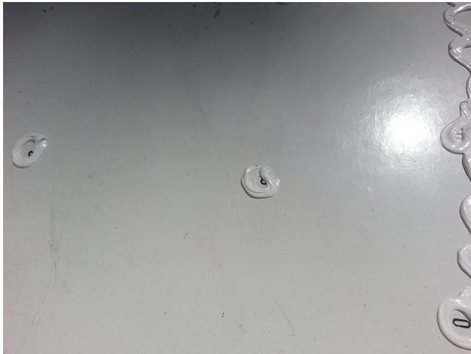
Figure 6 - Under Antenna Sealer
