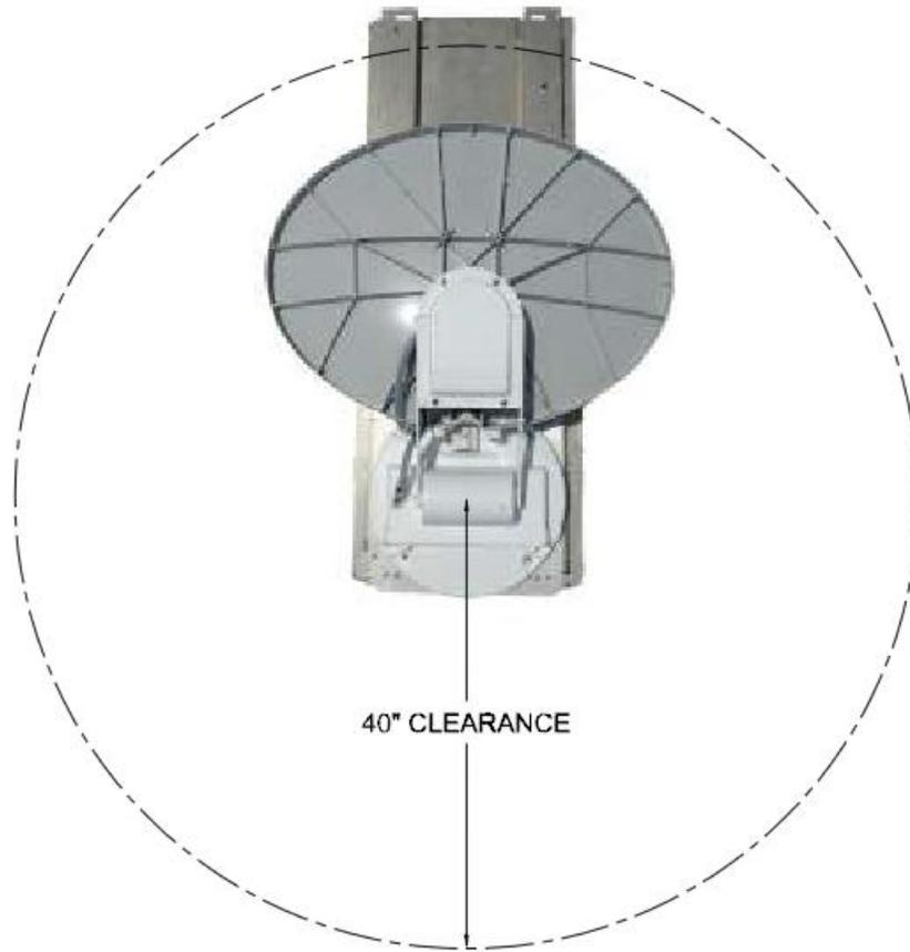
Figure 4 - Antenna Clearance
